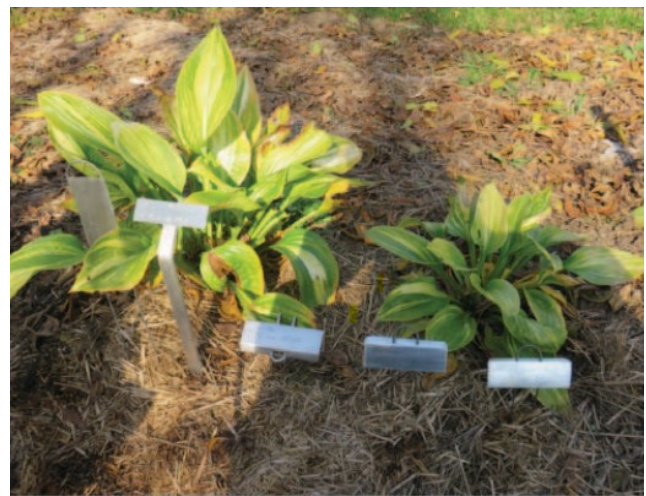
Plant stakes constructed of different materials (aluminum, stainless steel, and galvanized) were marked with a No. 2 pencil, then placed in the garden. The plant names were difficult to read because the pencil lead is so close to the same color as the metal.
